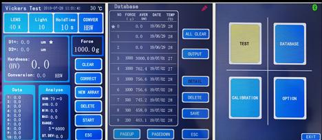
It can be used to determine the Vickers hardness of steel, non-ferrous metals, ceramics, treated layers of metal surface, and the hardness grads of carburized, nitrided and hardened layers of metals. It is also suitable to determine the Vickers hardness of micro and super thin parts.
